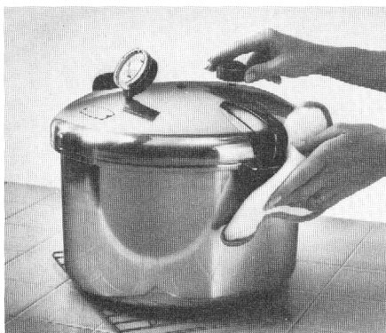
On canners with the spring-dial gauge, wait until the indicator returns to zero before removing the pressure regulator.
