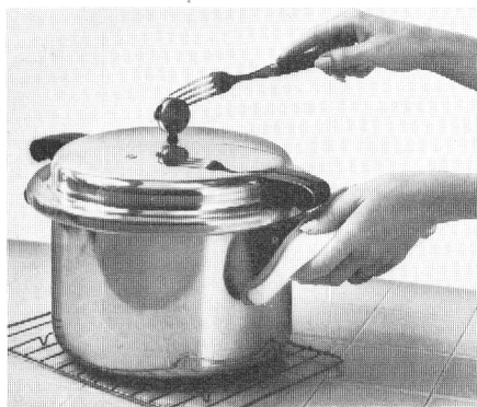
On canners with a weight gauge, let canner cool before nudging the gauge gently. If no steam is visible, lift off gauge.
